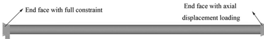
Fig. 4. Model for predicting elastic performance of racket handle with full constraint and displacement loading
